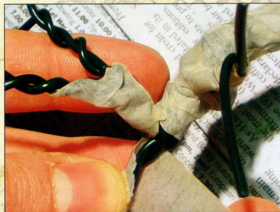
▲ COVERING THE GAPS Masking tape is a cheap and effective way to cover the bare wire.
