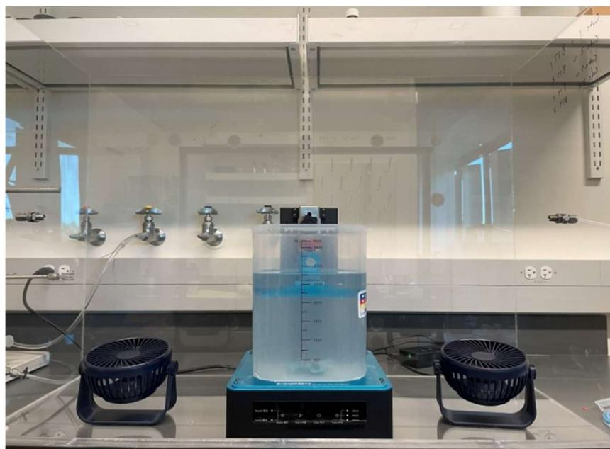
**Figure 24: Build plate transferred from the printer to the wash & cure.**
