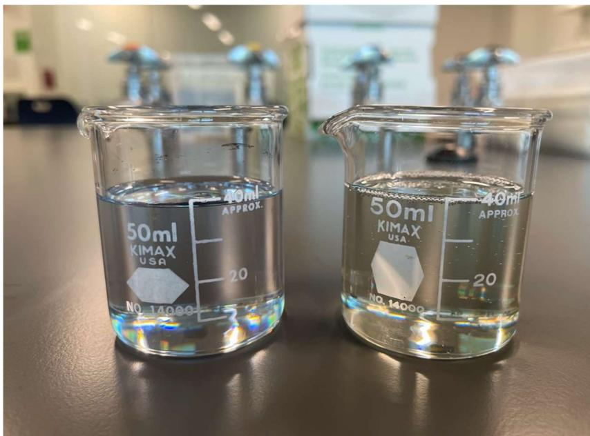
**Figure 22: Anycubic resins in beakers, oil-based on the left and plant-based on the right.**
