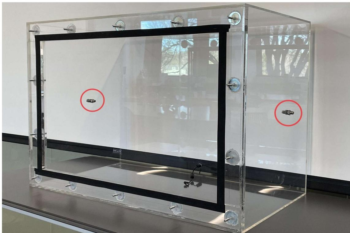
**Figure 16: Enclosure, 315 Liters. (.94m x .66m x .66m)**
