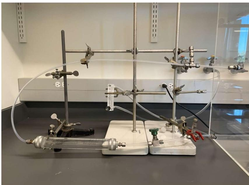
Figure 25: Swagelok manifold, flow path indicated.
